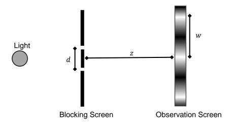
When the light is turned on, the observation screen has a repeating pattern of bright and dim fringes. The theoretical relationship between the distance between bright fringes (w), the separation of the slits (d) and the distance between the blocking screen and observation screen (z) is:
