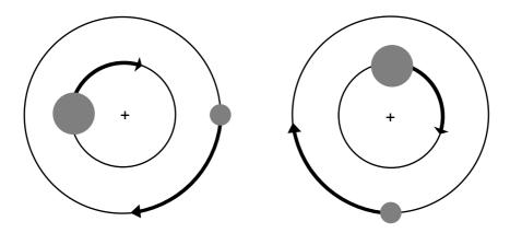
The two-body system diagrams above show that as the two bodies orbit the barycentre, their centres of mass are always radially opposite each other – each body has the same orbital period. Each body applies a gravitational force on the other, pulling it towards the barycentre. The bigger mass is always closer to the barycentre than the smaller mass.
