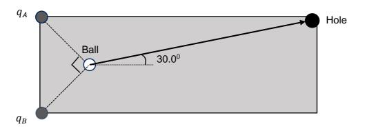
The charges  $q_A$  and  $q_B$  are located on the corners of the short edge of the putting area, equidistant from a golf ball. These charges share the same sign of charge as the golf ball, thus each repels the golf ball. Let the force acting on the golf ball due to charge  $q_A$  be called  $F_A$  and the force acting on the golf ball due to charge  $q_B$ ,  $F_B$ . Charge  $q_A$  is 260 nC and the golf ball has a 140 nC charge.
