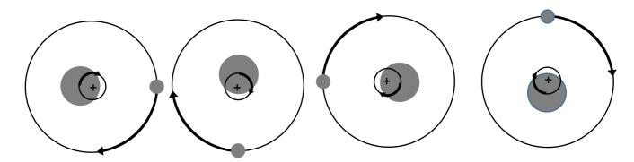
For these two-body system, the barycentre can be calculated from knowledge of the masses and total distance separating the two bodies:
